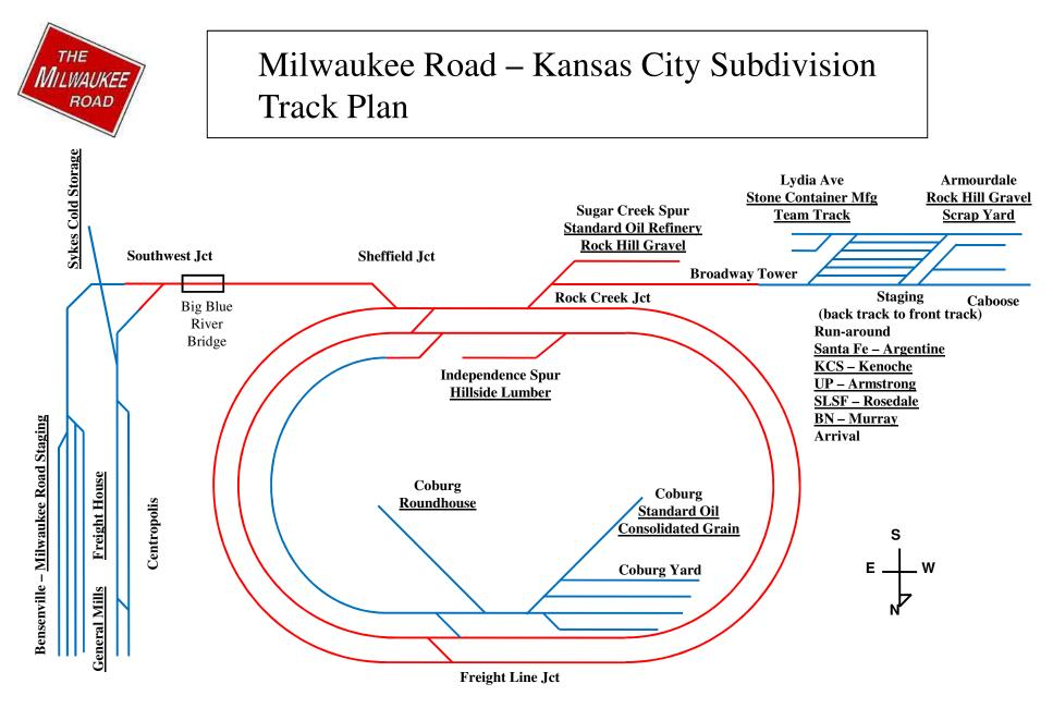
Legend: **Bold** text = Town / Location Name, <u>Underlined</u> text = Industry Name Eastward trains travel counter-clockwise on the loop. Westward trains travel clockwise. Red Lines = CTC Territory – Signals govern. Blue lines = Yard Limits – No signals, yard movement rules govern.
